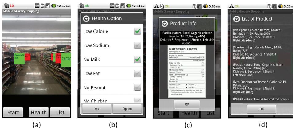
Fig. 8. Screenshot of (a) the AR mobile shopping app, (b) the health conditions selection screen activated by clicking the “Health” button, (c) the product information screen activated by clicking on an AR tag associated with a product, and (d) a typical non-AR grocery list used to compare against the AR UI (see evaluation in 5.4).
