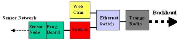
**Figure 6: A block diagram of our weather network. The webcam, soekris, and trango radio all connected to the switch via wired ethernet. The sensor node connected to the soekris via a USB-to-serial cable.**
