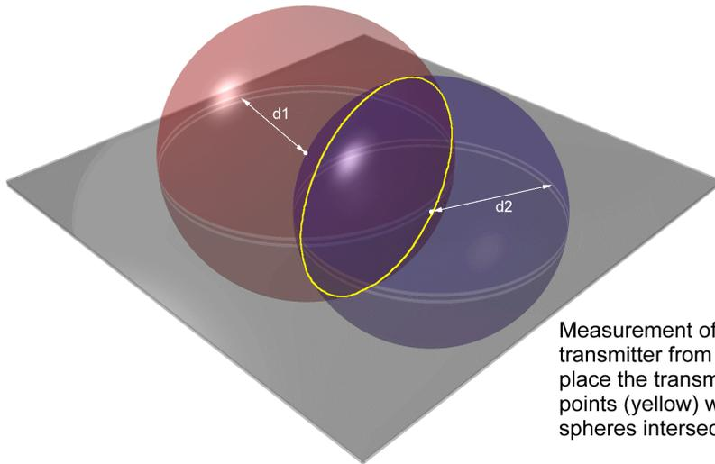
Measurement of distances  $d_1$  &  $d_2$  to the transmitter from two receivers allows us to place the transmitter on a circular locus of points (yellow) where the red and blue spheres intersect.
