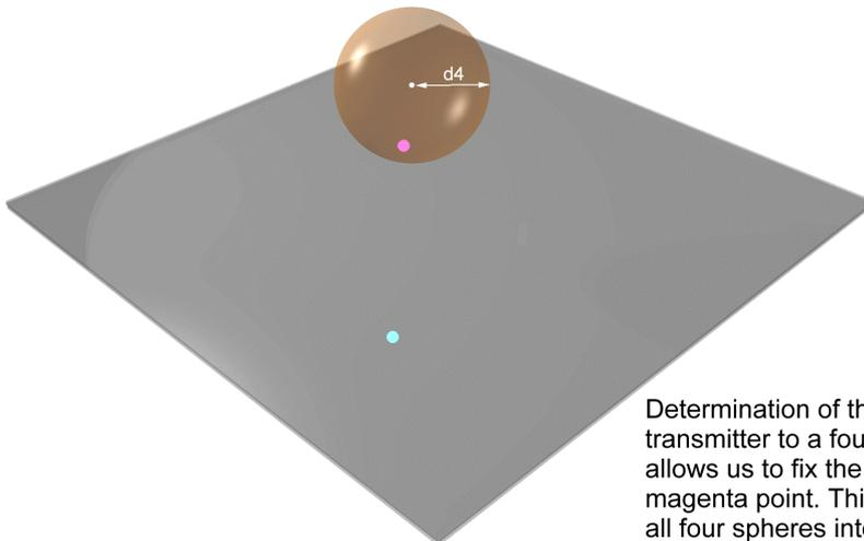
Determination of the distance  $d_4$  from the transmitter to a fourth, non-coplanar receiver allows us to fix the transmitter's location at the magenta point. This is the single point at which all four spheres intersect.
