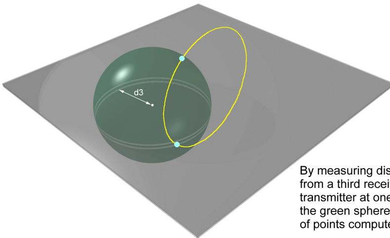
By measuring distance  $d_3$  to the transmitter from a third receiver, we can place the transmitter at one of two points (cyan) where the green sphere intersects the circular locus of points computed previously.
