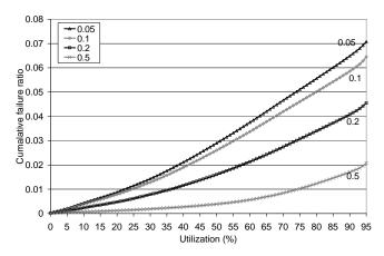
Figure 2: Cumulative failure ratio versus storage utilization achieved by varying the  $t_{pri}$  parameter and  $t_{div}=0.05$ .
