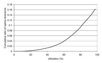
Figure 5: Cumulative ratio of replica diversions versus storage utilization, when  $t_{pri} = 0.1$  and  $t_{div} = 0.05$ .
