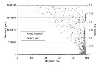
Figure 6: File insertion failures versus storage utilization for the NLANR trace, when  $t_{pri}=0.1$ ,  $t_{div}=0.05$ .
