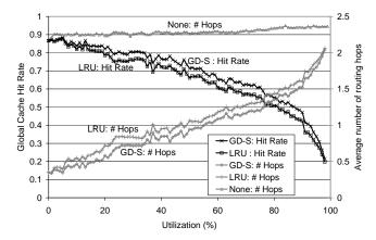
Figure 8: Global cache hit ratio and average number of message hops versus utilization using Least-Recently-Used (LRU), GreedyDual-Size (GD-S), and no caching, with  $t_{pri} = 0.1$  and  $t_{div} = 0.05$ .
