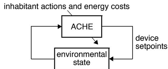
**FIGURE 2.** ACHE specifies device intensity setting (brightness), which affects the state of the environment, which in turn serves as input to ACHE. The training signals to ACHE are the actions taken by the inhabitants and energy costs.
