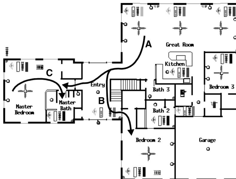
**FIGURE 6.** A floor plan of the adaptive house, including locations of sensors and actuators. Three trajectories are indicated by arrows labeled A, B, and C.
