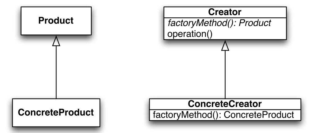
Factory Method leads to the creation of parallel class hierarchies; ConcreteCreators produce instances of ConcreteProducts that are operated on by Creator's via the Product interface 20
