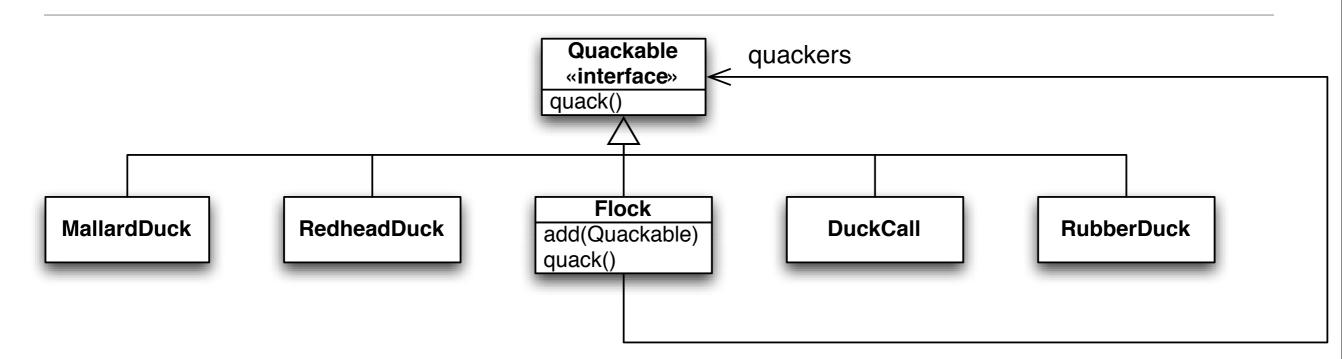
Note: Iterator pattern is hiding inside of Flock.quack(); **Demonstration**
