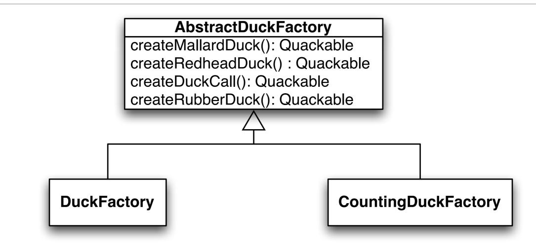
CountingDuckFactory returns ducks that are automatically wrapped by the QuackCounter developed in Step 4
