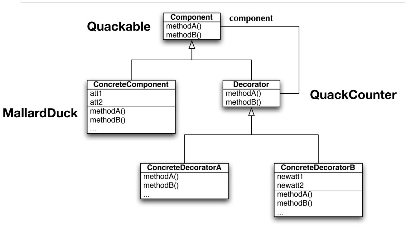
No need for abstract Decorator interface in this situation; note that QuackCounter follows ConcreteDecorators, as it adds state and methods on top of the original interface. <sup>12</sup>
