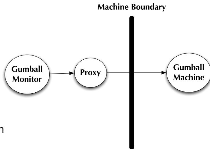
The Gumball Monitor talks to the Proxy object, thinking that its a Gumball Machine object. The Proxy communicates with the "real" Gumball Machine, and returns any results back to the monitor.
