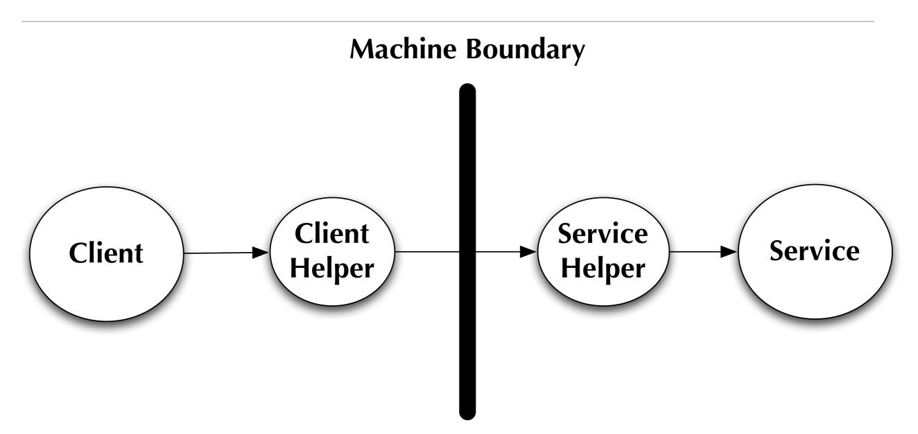
RMI creates "helper" objects that live on the client and service sides of a remote transaction. The client helper acts as a proxy for the remote service and sends method call information to the service helper. The service helper invokes the requested method on the service and returns the results.
