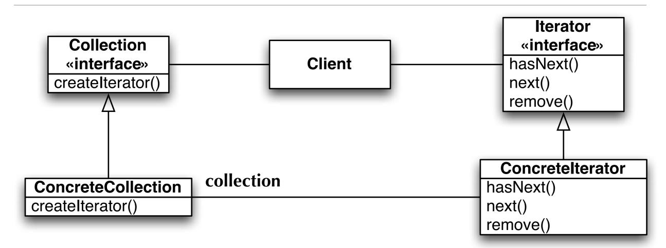
Each concrete collection is responsible for creating a concrete iterator. The Concretelterator has an association back to the original collection and keeps track of its progress through that collection.
