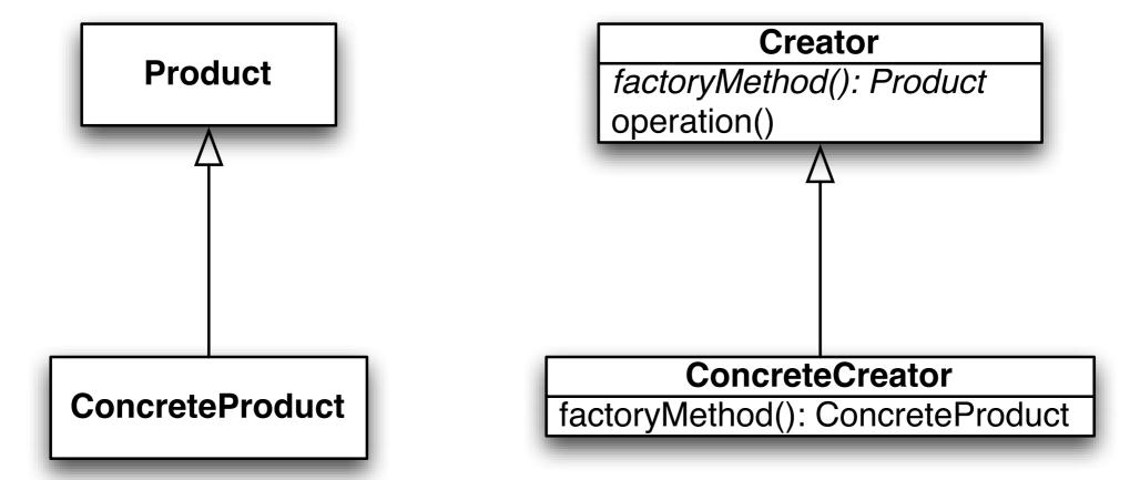
Factory Method leads to the creation of parallel class hierarchies; ConcreteCreators produce instances of ConcreteProducts that are operated on by Creator's via the Product interface
