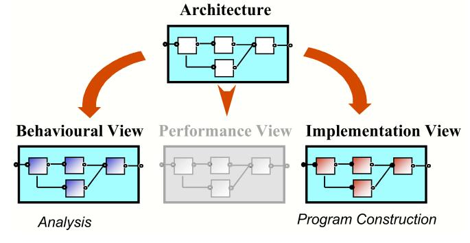
We consider that the models for analysis and the implementation should be considered as elaborated views of this basic design structure.
