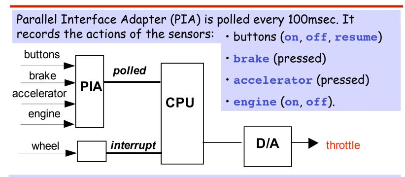
Wheel revolution sensor generates interrupts to enable the car **speed** to be calculated.
