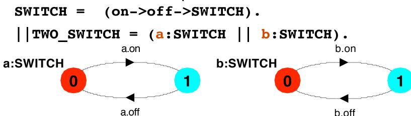
An array of instances of the switch process:
