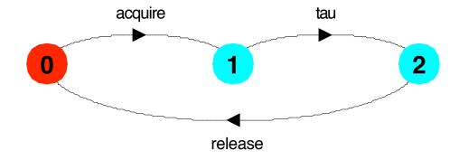
Minimization removes hidden tau actions to produce an LTS with equivalent observable behavior.
