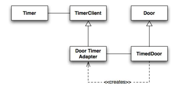
The solution is to keep the interfaces separate and make use of the adapter pattern to allow TimedDoor access to Timer and its functionality; note, here that this solution keeps TimedDoor independent of Timer and TimerClient
