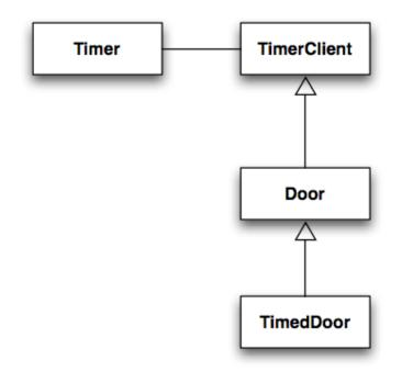
Here, Door is made to extend TimerClient so that TimedDoor can interact with the Timer object. Unfortunately, now all subclasses of Door depend on TimerClient even if they don't need Timing functionality!
