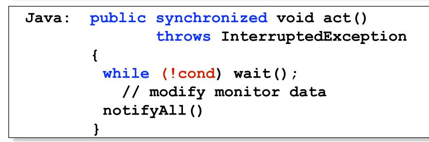
The **while** loop is necessary to retest the condition *cond* to ensure that *cond* is indeed satisfied when it re-enters the monitor.
