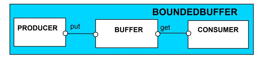
The behaviour of BOUNDEDBUFFER is independent of the actual data values, and so can be modelled in a dataindependent manner.
