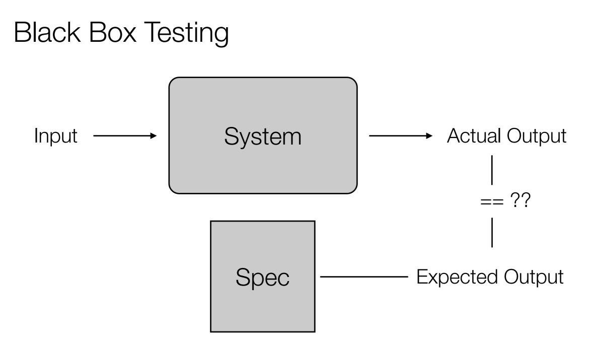
A black box test passes input to a system, records the actual output and compares it to the expected output
