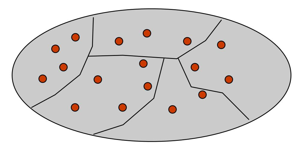
The testing literature advocates folding the space into equivalent behaviors and then sampling each partition
