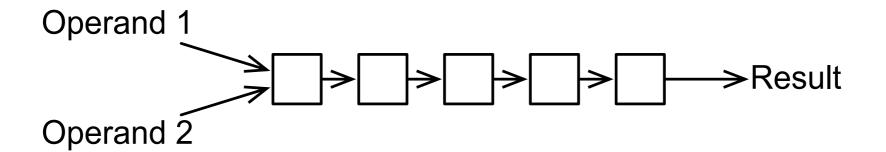
• In this example, if each step takes one clock cycle, it would take 5 clock cycles to perform the multiplication
