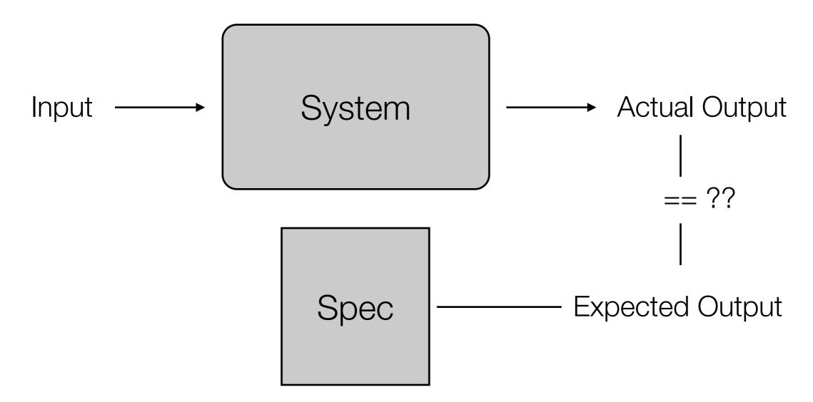
A black box test passes input to a system, records the actual output and compares it to the expected output
