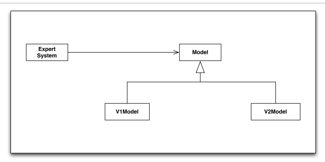
We want to provide the expert system with a single model that it understands; we will subclass this model to integrate the different versions of the CAD system
