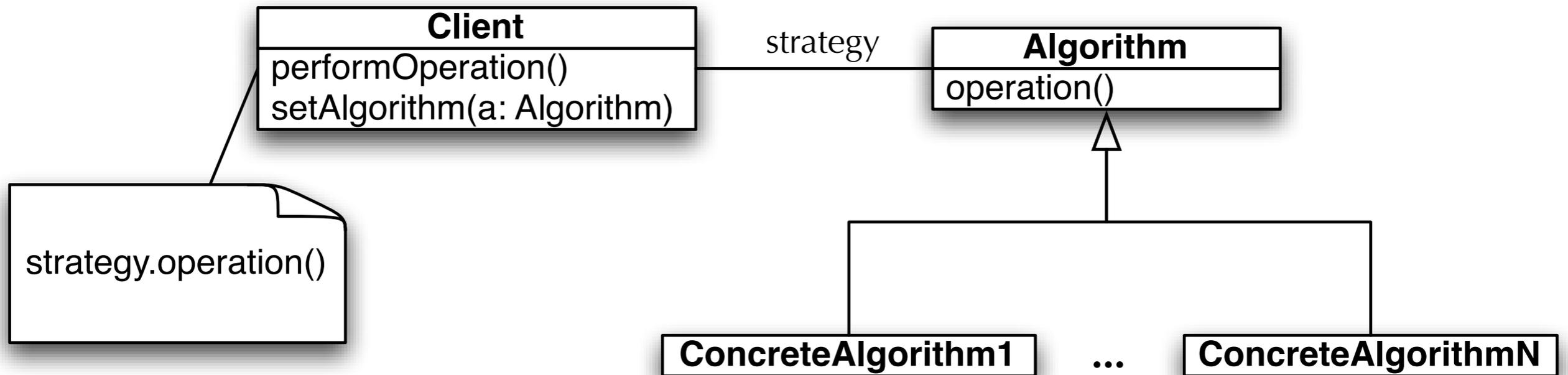
Algorithm is pulled out of Client. Client only makes use of the public interface of Algorithm and is not tied to concrete subclasses.
