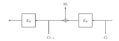
Figure 1: CBC Mode Decryption. Fixing  $C_{\ell}$  and flipping any bit of  $C_{\ell-1}$  flips the corresponding bit of  $M_{\ell}$ .
