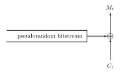
Figure 3: Stream-Based Decryption. Similar to CBC, flipping bits in  $C_{\ell}$  flip the corresponding bits in  $M_{\ell}$  independent of the key stream used for decryption.
