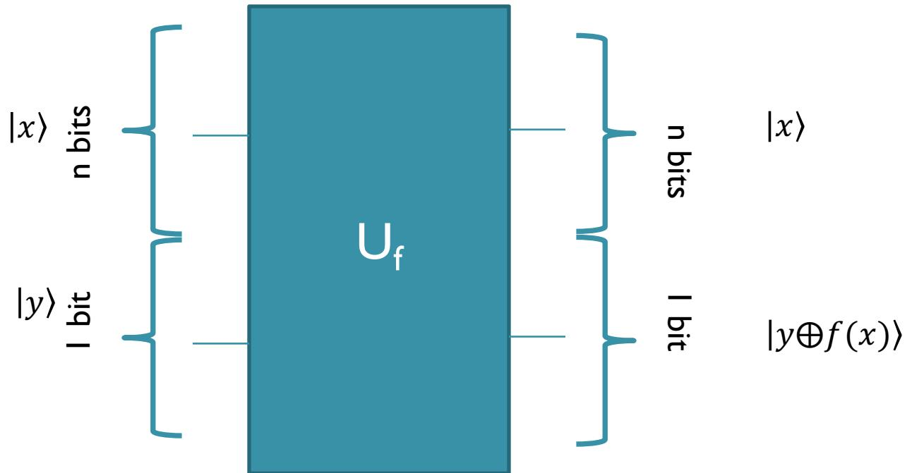
$U_f$  applied to the computational basis state  $|x\rangle_n|y\rangle_1$  flips the value  $y$  of the output register iff  $f(x)=1$ .
