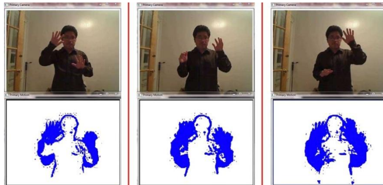
Figure 3. Visible images (top) and binary versions of corresponding motion history images (bottom)
