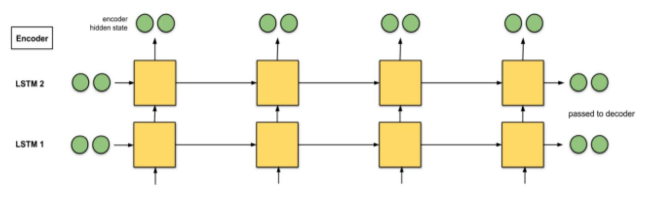
Luong's method encodes input with a 2-layer stacked LSTM
