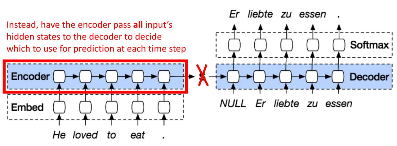
Decoder decides which inputs are needed for prediction at each time step; e.g., "hard attention" focuses on one input
