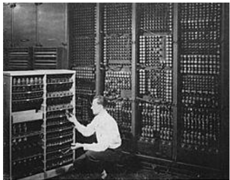
(ENIAC’s vacuum tubes being changed)
