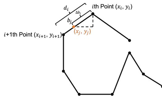
Figure 10: The schematic of computing the equidistant points.
