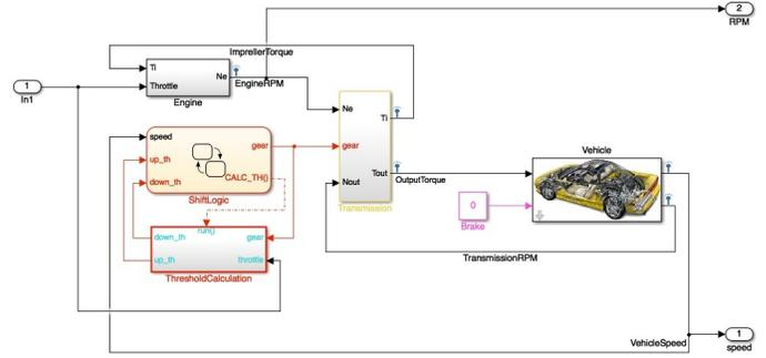
Figure 1: The automatic transmission system Simulink<sup>®</sup>/Stateflow<sup>™</sup> model.
