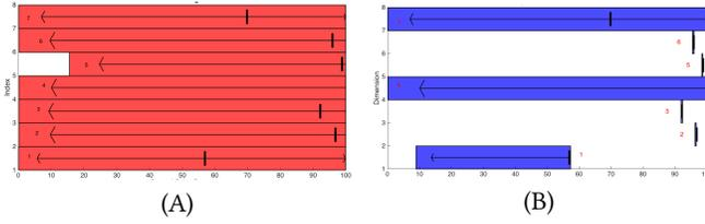
**Figure 3: (A) The tornado diagram showing the range for each input control point in isolation, and (B) The falsification neighborhood. The x-axis represents the range of control points  $[0, 100]$  and the y-axis represents indices 1 to 7.**
