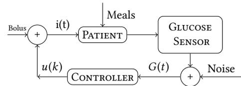
**Figure 7: Closed loop diagram for the artificial pancreas control scheme taken from Cameron et al [10].**
