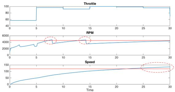
Figure 2: Counter-example for  $\phi_1$  found by S-Taliro with the responsible portions of the output traces highlighted.
