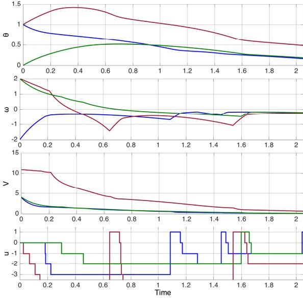
**Figure 5: Simulation of the Closed Loop System for Inverted Pendulum. States, Lyapunov function and control input are shown for each trace with different colors.**
