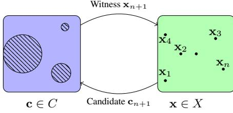
**Figure 3: Illustration of the CEGIS iteration, showing the space of candidates, witnesses and the iterative synthesis process.**
