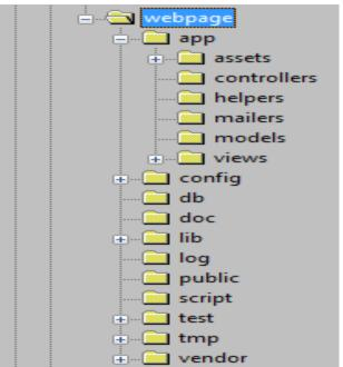
These are the files which rails automatically generates to create the framework for our application.
